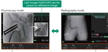
Exposure conditions can be operated on the console
