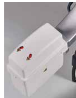
Zero dose centering with laser localizers on X-ray tube and flat panel detector.
