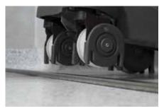
Easy lift front wheels safely navigate over cords and floor transitions.
